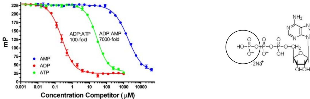
The Transcreener™ monoclonal antibody is a novel anti-ADP antibody that can distinguish between a single phosphate group. Antibody/Tracer complex was mixed with increasing concentrations of ATP, ADP, or AMP to generate the competition curves. The anti-ADP mAb is 100-fold and 7000-fold more selective for ADP, relative to ATP or AMP. The EC<sub>50</sub> values for ADP, ATP, and AMP are 0.25 μM, 27.8 μM, and 1800 μM, respectively.
