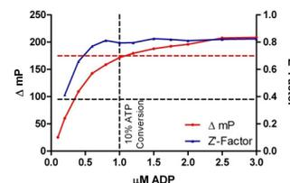
**Figure 4. EnVision passes validation with ADP<sup>2</sup> assay without modifications to protocol.** The validation criteria include: Z' ≥ 0.7 at 10% conversion of 10 μM ATP, a Δ mP shift ≥ 95 mP at 10% conversion and read time ≤ 5 minutes. Z' = 0.79 with Δ mP shift of 172 was achieved with 2 nM tracer at 10% ATP conversion with 30 flashes and read time of 1 minute, 20 seconds.
