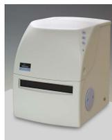
**Figure 2. The EnVision HTS Multilabel Plate Reader.** The EnVision is capable of reading 96, 384, and 1536-well assay plates. Filters and dichroic modules are interchangeable and easy to install. The simultaneous dual-detection capabilities of the reader enable fast read times. For far red FP, we used the following: optimized Cy5 FP Dual Emission Label, 620/40 nm excitation filter, 688/45 nm emission filter, and D658/1p688 dual mirror.
