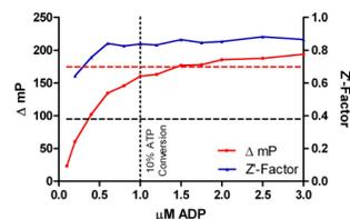
**Figure 3. The Safire<sup>2</sup>™ meets BellBrook Labs' Instrument Validation Criteria.** The validation criteria include:  $Z' \geq 0.7$  at 10% ATP conversion of 10 μM ATP, a  $\Delta mP$  shift  $\geq 95$  mP at 10% conversion and read time  $\leq 5$  minutes. The assay passed validation under the following conditions: 1 flash per well, 50 ms delay between move and read, resulting in a  $Z' = 0.84$ ,  $\Delta mP$  of 161 in 57 seconds.
