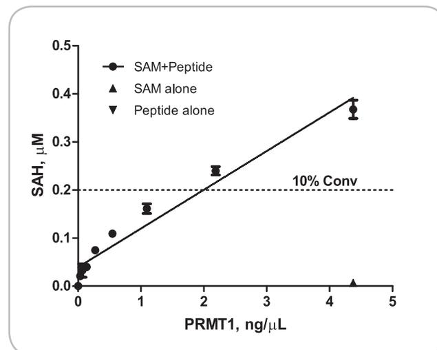
Figure 4. Linear relationship between PRMT1 concentration and SAH formation. The polarization values were converted into SAH (product formed) using a standard curve set up under similar conditions.
