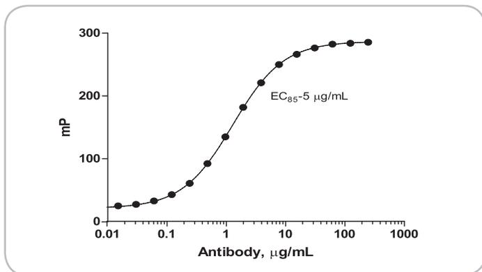
Figure 2. AMP<sup>2</sup>/GMP<sup>2</sup> antibody titration in the presence of 2 µM SAM and 10 µM H4 (1-20) peptide. An optimal concentration of 5 µg/mL was determined based on this titration.
