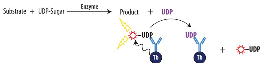
**Figure 1. Schematic overview of the Transcreener® UDP<sup>2</sup> TR-FRET Red Assay.** The Transcreener® UDP Detection Mixture contains a UDP HiLyte647 tracer bound to a UDP<sup>2</sup> antibody conjugated to terbium (Tb). Excitation of the Tb complex in the UV range (~330 nm) results in energy transfer to the tracer and emission at a higher wavelength (665nm) after a time delay. UDP produced by the target enzyme displaces the tracer, which causes a decrease in TR-FRET.
