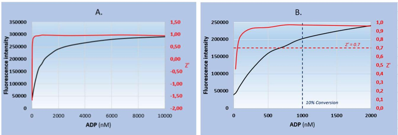
*Figure 3. . A). Z' values (red line) and fluorescence intensities (black line) observed in a standard curve mimic conversion of 10 µM ATP to ADP. B). Zoomed view of the 0-2000 nM ADP section of the standard curve shows the Z' validation minimal qualification data (red dotted line) and 10% ATP conversion validation point (blue dotted line).*
