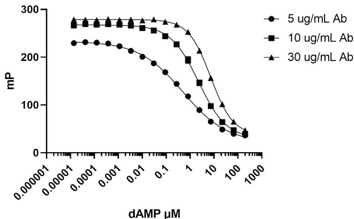
Standard curves illustrate tuning the assay to the appropriate levels for the sensitivity desired. In this example 200  $\mu\text{M}$  dAMP standard curves were completed using 5, 10, and 30  $\mu\text{g/mL}$  final concentrations of dAMP antibody. Using the correct dAMP antibody for the amount of dAMP produced in the assay is imperative to achieving quality results. Use the following equations to calculate the Z' factor:
