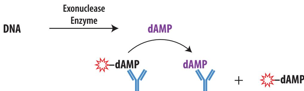
**Figure 1. Schematic overview of the Transcreener dAMP FP Assay.** The Transcreener dAMP Detection Mixture contains an dAMP AlexaFluor® 633 tracer bound to an dAMP antibody. dAMP produced by an exonuclease enzyme displaces the tracer, which rotates freely, causing a decrease in FP.
